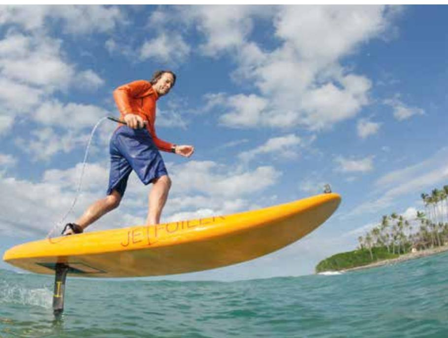
Don Montague, a former professional windsurfer, will teach you how with the help of Kai Concepts. To be able to do so, they have created *Jetfoiler*, a surfboard that combines an electrical engine with a hydrofoil. This electrical "magic carpet" raises slightly above the water surface, making you feel as if you are surfing even when there are no waves at all with no sound nor trail behind you!
